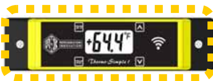
Flashing Yellow – Over Temp. Alarm (Or only the first 60 minutes of Alarm with Red Alarm option)
