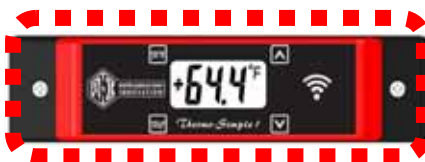
OPTIONAL Flashing Red – Over Temp. Alarm (After the first 60 minutes of an Amber alarm)
