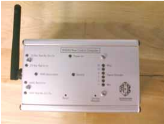
Figure 1-8: Row Control Computer (RCC).
