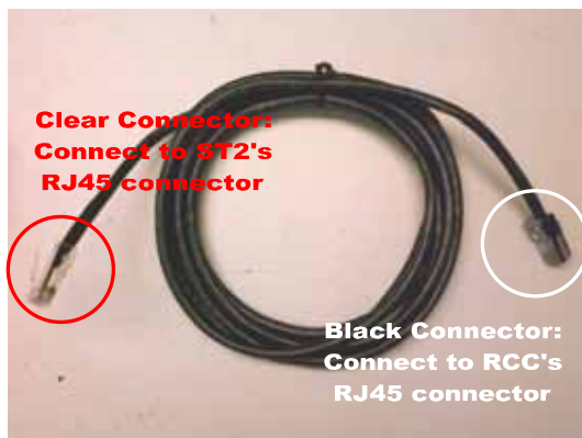
Figure 1-7: RCC to Spine Communication Cable.
